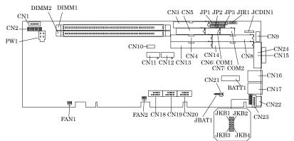
Figure 2.1. Connector & Jumper Location
